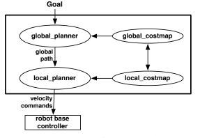
Fig. 1: Concept of navigation methods (www.ros.org/wiki/move\_base)
