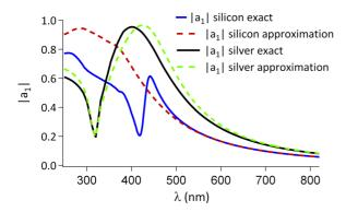
FIG. 1. Mie coefficient  $|a_1|$  plotted with respect to the wavelength in the case of a sphere of radius 60 nm made of silicon [25] and silver [26]. Full lines: calculated with the exact expression derived in Eq. (1) with n=1 with silicon (blue) and silver (black). Dashed lines: approximation  $a_1^{(T1)}$  in Eq. (24) taken from Ref. [15] in red for silicon and green for silver.
