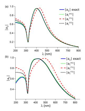
FIG. 4. Comparison between exact (full blue line) and approximations (23) (dotted green line) and (24) (dashed red and black lines) of  $a_1$  for a sphere of silver [26] 60 nm (a) and 80 nm (b) in radius.
