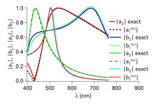
FIG. 6. Comparison between exact calculations and approximations 23 for  $a_1$  (full red line and dashed black line),  $b_1$  (full blue line and dotted green line),  $a_2$  (full green line and dashed gray line), and  $b_2$  (full cyan line and dotted red line) for TiO<sub>2</sub> [41] 140 nm in radius.
