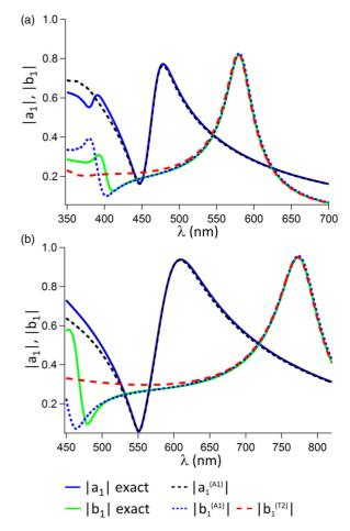
FIG. 5. Comparison between exact calculations of  $a_1$  (full blue line) and  $b_1$  (full green line) with approximations (23) of  $a_1$  (dashed black line) and  $b_1$  (dotted blue line) and power-series approximations of  $b_1$  (24) (dashed red line), for a sphere of silicon [25] of radius 70 nm (a) and 100 nm (b).
