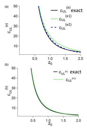
FIG. 7. Comparison between the exact  $\varepsilon_{UL}$  (black full line) required to reach the resonance and the prediction provided by Eqs. (15) and (16) respectively labeled  $\varepsilon_{UL}^{(e1)}$  and  $\varepsilon_{UL}^{(h1)}$  (dotted green line). A better approximation of  $\varepsilon_{UL}^{(e)}$  is obtained by solving  $\varphi_n^{(W1)}(z_s) = -n\varepsilon_s$ , labeled  $\varepsilon_{UL}^{(e2)}$  (dashed blue line)
