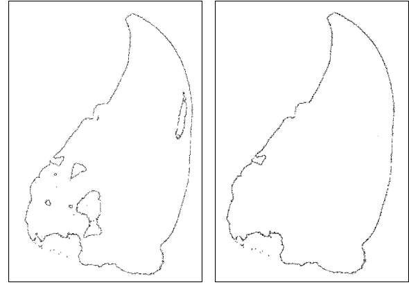
(a) Contours identified by the Canny algorithm. (b) Contour selected by post-processing.
