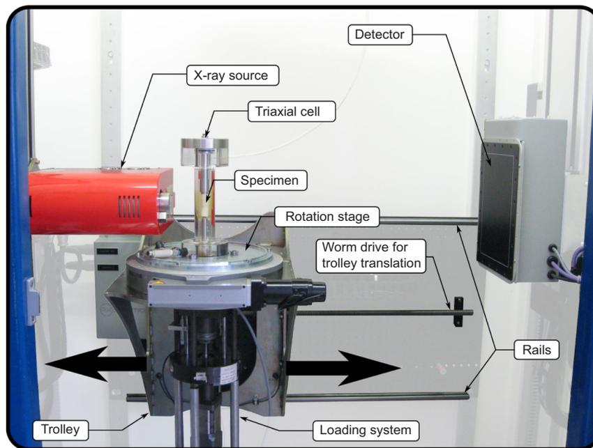
**Fig. 1.** Laboratoire 3SR x-ray scanner. The background is faded out for clarity; blue edges visible left and right are the cabin door frame
