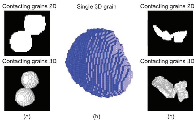
**Fig. 3.** (a) Two-dimensional (2D) and 3D views of two glass ballotini in contact (these particles are close to spheres). (b) 3D view of a single Caicos ooid, with its jagged, voxelised nature underlined (courtesy of J. Andrade). (c) 2D and 3D views of two Hostun sand grains in contact
