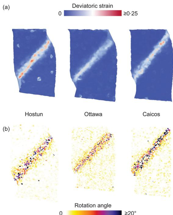
**Fig. 2.** Measurements made on increments in the residual stress state of Hostun sand, Ottawa sand and Caicos ooid tested in triaxial compression at 100 kPa confinement. The fields plotted are deviatoric shear strain (a) and the intensity of 3D grain rotation (b). Note that the strain increments are not the same: the one for Hostun sand is particularly larger than the rest
