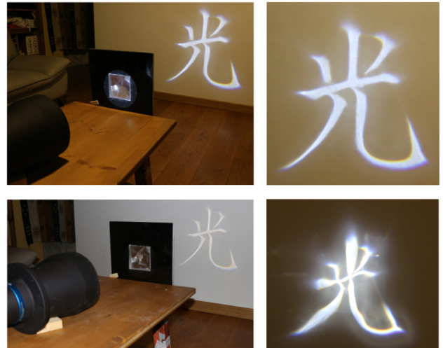
Figure 18: Stability with respect to the depth of the focus plane. The lens of HIKARI is designed to focus at a distance of 2 meters. The target screen is at different depths, top: 1.5 meters; bottom: 1m (left), 50cm (right).
