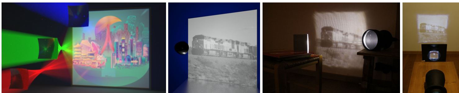
Figure 1: Our algorithm can be used to design mirrors and lenses that reflect or refract collimated or point light sources onto a prescribed distribution of light. From left to right: Three lenses that refract the three channels of a color image; Mirror that reflects a point light source (located inside the mirror); Fabricated mirror that reflects a collimated light source; Fabricated lens that refracts a collimated light source.
