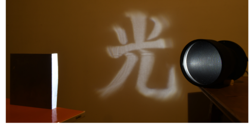
Figure 17: Fabricated mirror for a collimated light source. HIKARI target.
