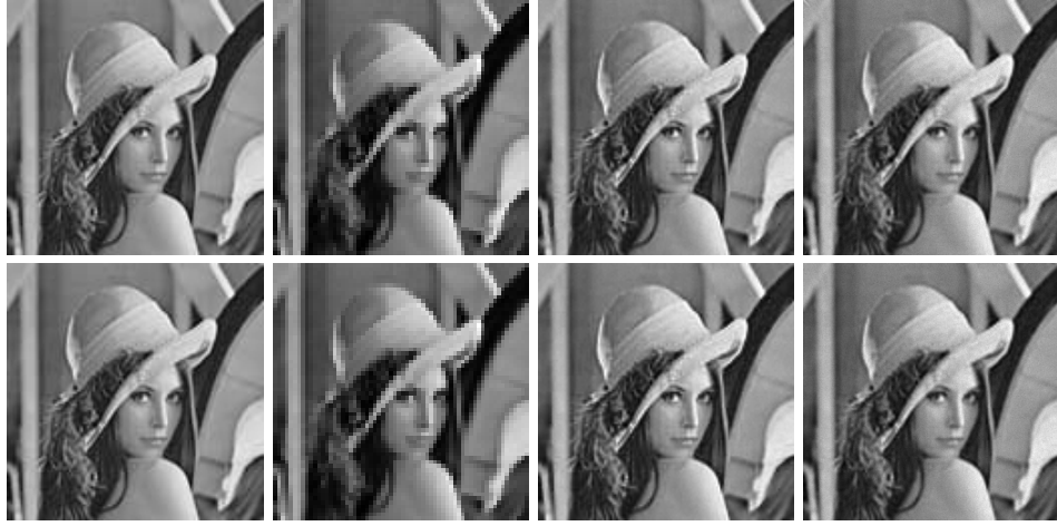
FIGURE 10. Comparison for different discretizations. Comparison of the forward simulations for the Point Source Mirror (first row) and Collimated Source Lens (second row) problems with different discretizations of the same target distribution. The dimensions of the original image (left) are 128x128. Then from left to right, the discretizations are the following: 64x64, 128x128, 256x256.
