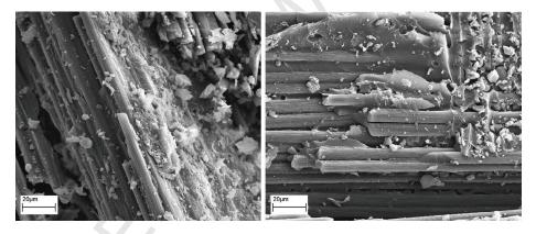
Figure 7: SEM visualization of carbon-phenolic material before (left) and after (right) the TG experiment under inert conditions and heating rate of 15  $^{\circ}C/min$ .
