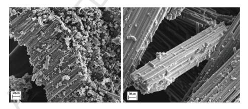
Figure 6: SEM visualization of carbon-PEKK crashed sample before (left) and after (right) the TG experiment under inert conditions and heating rate of 15  $^{\circ}C/min$ .
