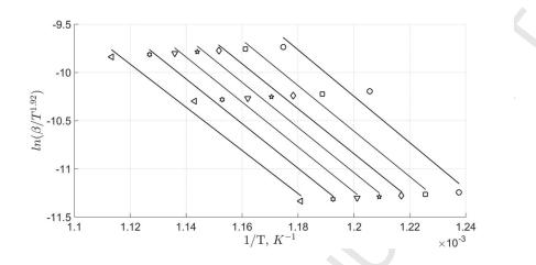
Figure 3: Example of Arrhenius-type plot for activation energy estimation with Starink method [47]. The slope of linear regression on the experimental data couples (dots) of three different beta corresponds to  $E_{\alpha,i}$ .
