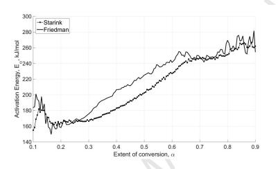
Figure 10: Activation energy vs. extent of conversion estimated by isoconversional methods for carbon-phenolic in inert atmosphere.
