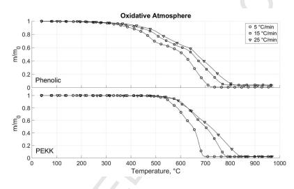
Figure 8: Mass loss curves obtained for  $\beta$  equal to 5, 15 and 25 °C in oxidative atmosphere. Comparison between carbon-phenolic and carbon-PEKK.
