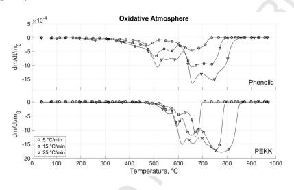
Figure 9: DTG curves obtained for  $\beta$  equal to 5, 15 and 25 °C in oxidative atmosphere. Comparison between carbon-phenolic and carbon-PEKK.
