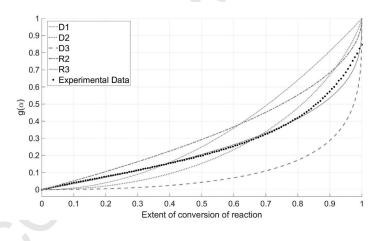
Figure 14: compensation effect method for decomposition model evaluation: carbon-PEKK in inert atmosphere, with regard to Starink activation energy estimated values.
