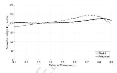
Figure 11: Activation energy vs. extent of conversion estimated by isoconversional methods for carbon-PEKK in inert atmosphere.
