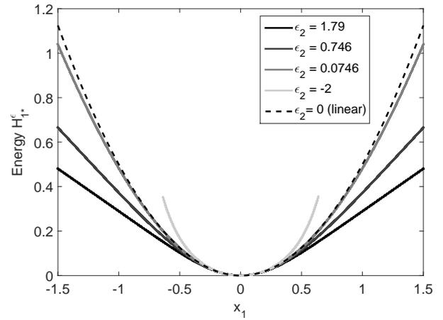
Figure 7:  $H_{1*}^\epsilon$  energies of the controlled system for different values of control parameter  $\epsilon_2$ .
