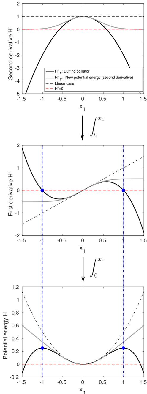
Figure 2: Second derivative, first derivative of potential energy and potential energy obtained by successive integrations with respect to the displacement  $x_1$ , represented in the case of the Duffing oscillator, the new well-posed energy, and the linear case. Red dot line represents the null energy level, and blue dot line indicates the coincidence between the turning points of the potential energy and the zeros of its first derivative.
