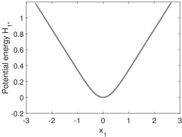
Figure 5: Potential energy  $H_{1*}$  as a function of the displacement  $x_1$  resulting from simulations of the new well-posed system for an input force  $f_0 = 2 \cdot 10^8 > f_{max} = 9.5 \cdot 10^7$ .
