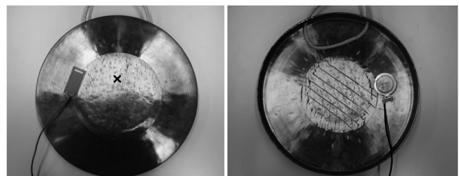
FIG. 6. Top view of the xiaoluo showing the location of the MFC sensor (left panel) and the electrodynamic actuator (right panel). The black cross shows the location of the mallet strike.
