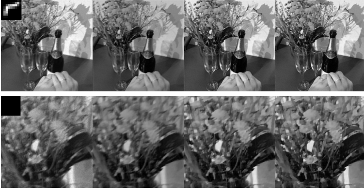
FIGURE 6. Deblurring with total variation regularization with Poisson noise and unknown boundaries. Results after 100 epochs. Top: From left to right: Blurry and noisy data with kernel (magnified), PDHG, DA-PDHG and DA-SPDHG (importance sampling, 3 subsets). Bottom: Close-ups of top row.
