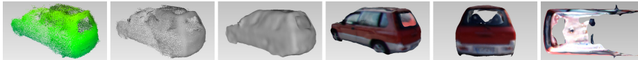
Fig. 2: Illustration of 3D Reconstruction Enhancement: from left to right are raw registration, smoothed point cloud, surface reconstruction, textured mesh in side view, back view and top view, respectively.
