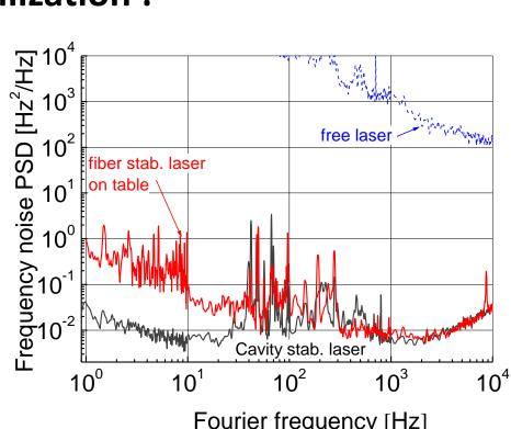
Frequency noise of laser stabilized onto 1-km fiber with passive spool isolation
