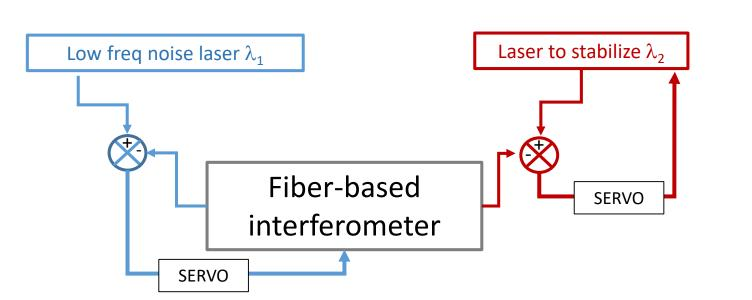
Same principle than transfer cavity but with fiber based interferometer
