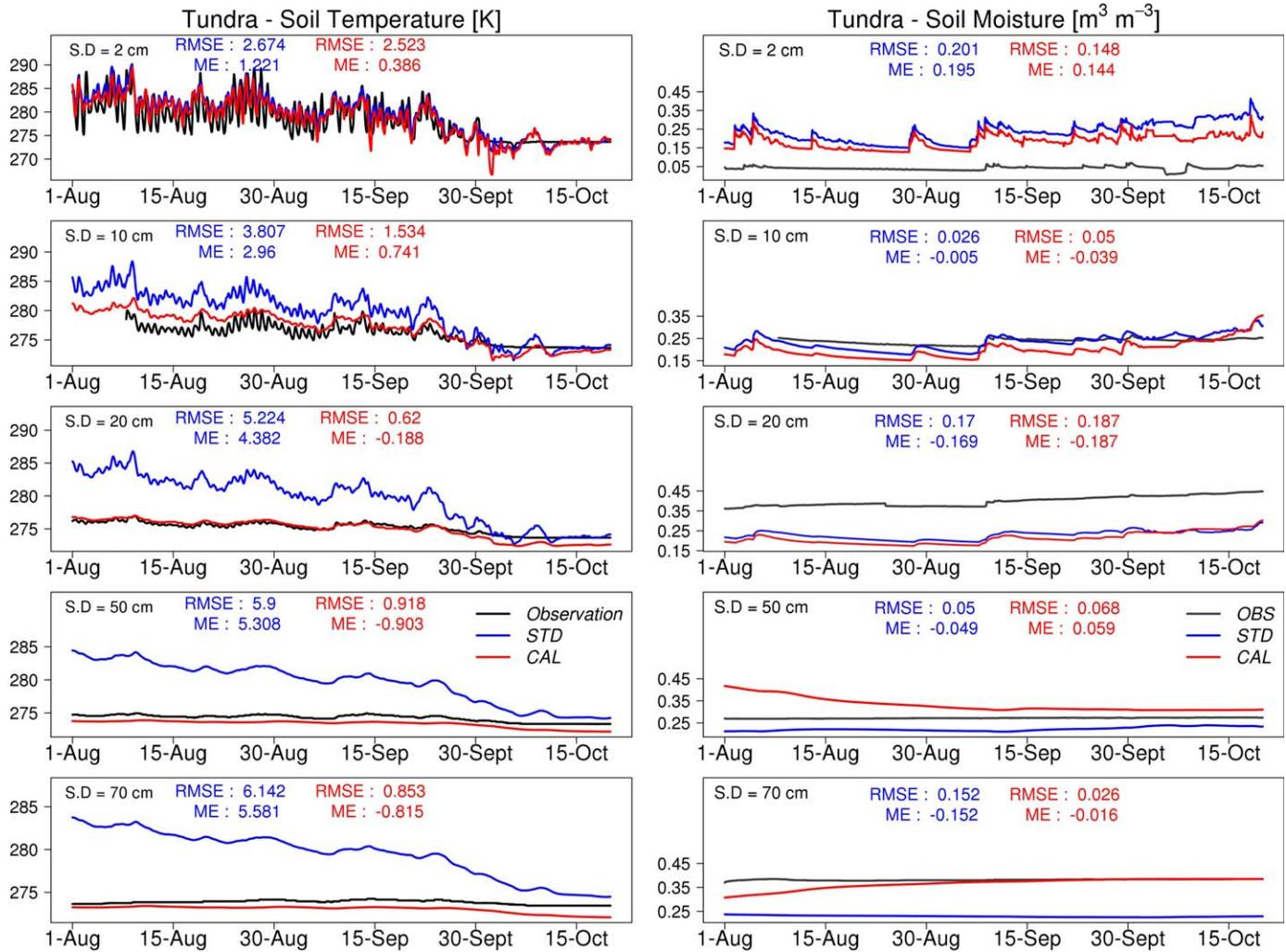
**Figure 8.** Comparison of simulated soil temperature (K) and soil moisture ( $\text{m}^3 \text{m}^{-3}$ ) at different soil depths (S.D.: 2, 10, 20, 50, and 70 cm) for the Tundra site. The standard (STD, in blue) and calibrated (CAL, in red) ORCHIDEE simulations are plotted against observations (in black). RMSE and bias (mean error; ME) are indicated in the corresponding color.
