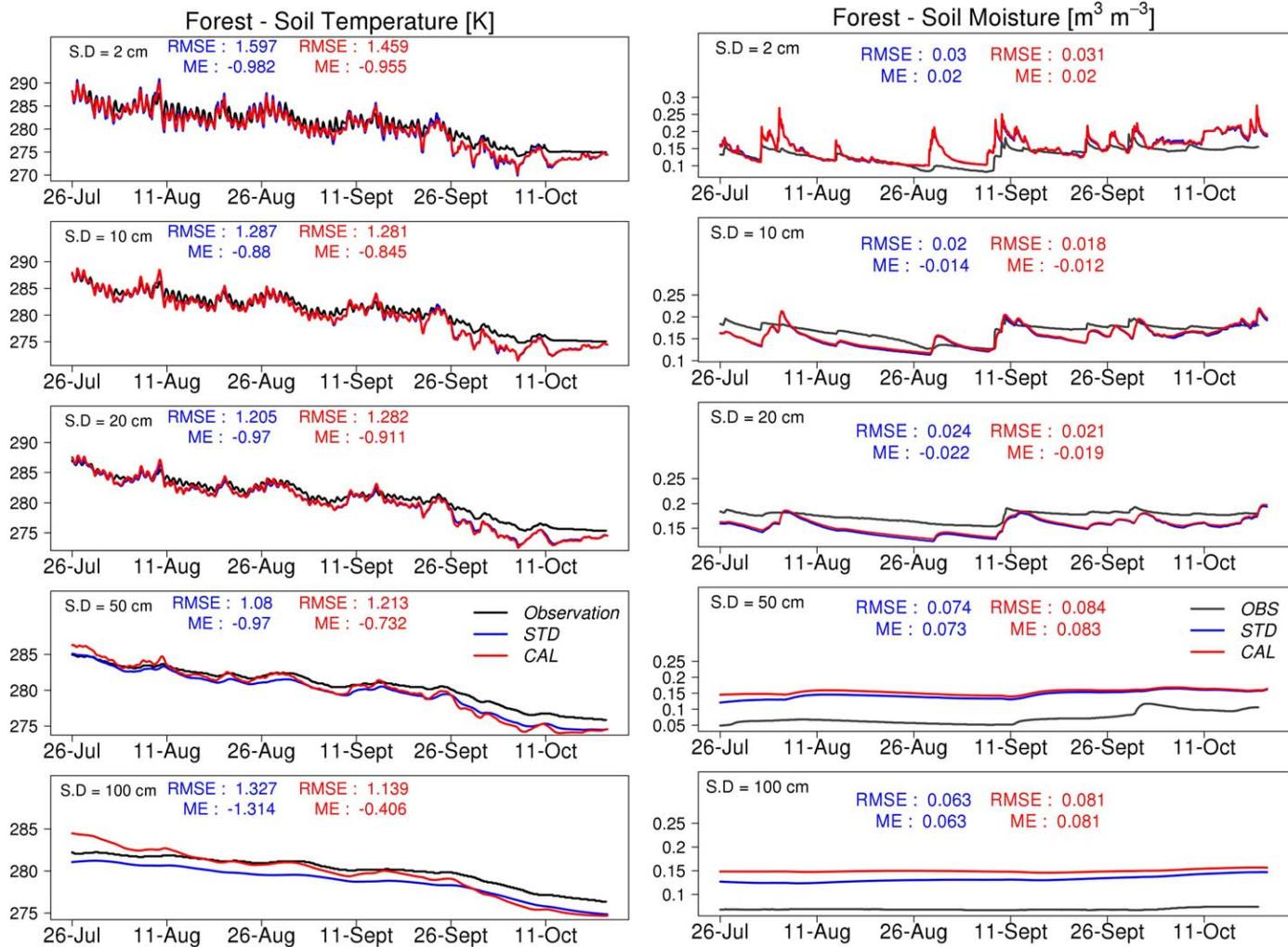
**Figure 7.** Comparison of simulated soil temperature (K) and simulated soil moisture ( $\text{m}^3 \text{m}^{-3}$ ) at different soil depths (S.D.: 2, 10, 20, 50, and 100 cm) for the Forest site. The standard (STD, in blue) and calibrated (CAL, in red) ORCHIDEE simulations are plotted against observations (in black). RMSE and bias (mean error; ME) are indicated in the corresponding color.
