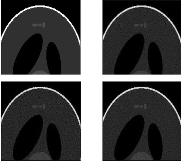
Fig. 6: Slice comparison between the original volume (top left) and JMAP reconstructed volumes  $St$  (top right),  $NiG$  (bottom left),  $VG$  (bottom right).  $64^3$  phantom size, 128 projections, SNR=30dB
