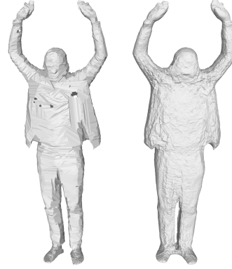
Figure 3. Left: the Confidence Volume with \alpha = \beta = 54 , equivalent to the Visual hull with the 54 cameras that see the subject; Right: the Confidence Volume with \alpha = \beta = 10 .
