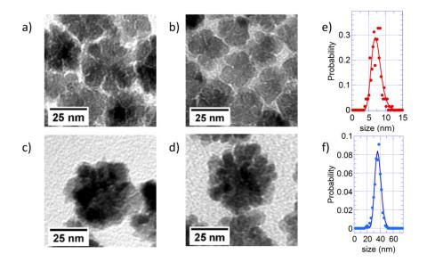
**Figure 2.** High magnification (HM) TEM micrographs of  $\gamma$ -Fe<sub>2</sub>O<sub>3</sub> nanoflowers: a) 36ff, b) 35ff, c) 30ff, and d) 15ff. Distribution of e) grain sizes of the 15ff batch (7.4±1.4 nm), and f) outer diameter (36.9±4.8 nm), measured on HM-TEM micrographs and log-normal fits.
