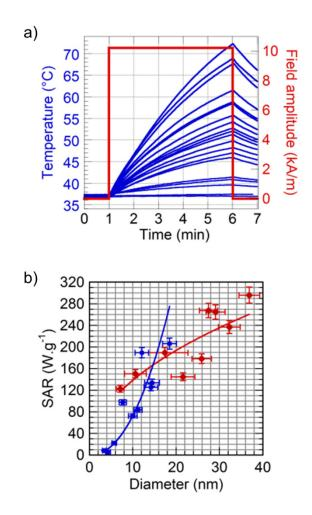
**Figure 4.** a) Temperature profiles *vs.* time of different samples of iron oxide concentration set at 3 g·L<sup>-1</sup>, under application of an AMF at  $H_{app}$ =10.2 kA·m<sup>-1</sup> and *f*=755 kHz. The full list of samples and corresponding initial slopes (within first 5 s) is given, on **Table S1**; b) Deduced *SAR vs.* mean diameter (determined by TEM) for smooth nanospheres (blue) and nanoflowers (red). Solid lines are power law fits of exponents 2.2 and 0.48, respectively.
