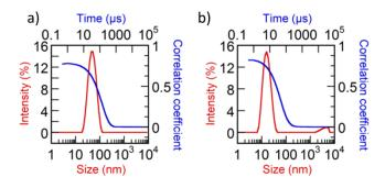
**Figure 3.** DLS correlograms and intensity-averaged distribution of diameters of a) 35ff nanoflowers ( $D_h$ =36 nm, PDI=0.13), and b) 20ff UUSPIO smooth spheres ( $D_h$ =16 nm, PDI=0.21). Values in parentheses correspond to the *Z*-average hydrodynamic diameter ( $D_h$ ,) obtained from the 2<sup>nd</sup> order cumulant fit, and polydispsersity index (PDI). See all DLS plots on **Figure S5**.
