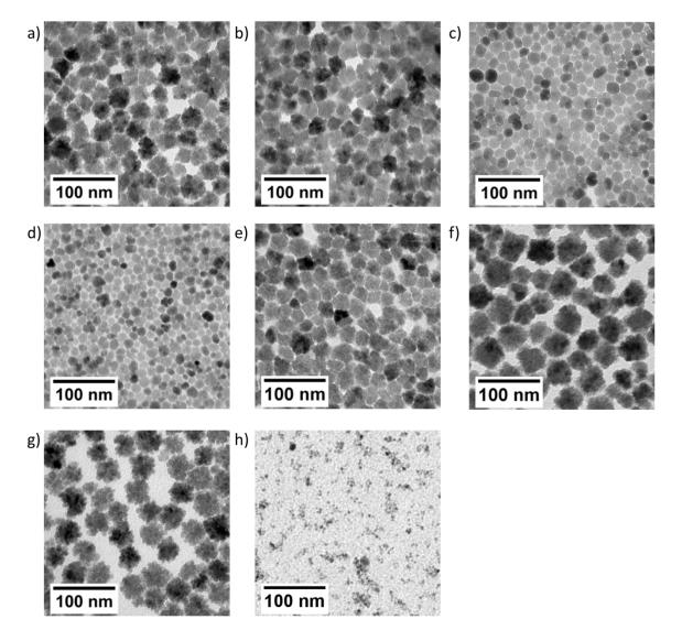
Figure 1. TEM micrographs of  $\gamma$ -Fe<sub>2</sub>O<sub>3</sub> NPs of mono- or multi-core morphology: a) 36ff (32.3±5.0 nm), b) 35ff (29.1±4.4 nm), c) 34ff (18.5±3.2 nm), d) 32ff (14.5±3.4 nm), e) 31ff (27.5±4.2 nm), f) 30ff (46.9±8.5 nm), g) 15ff (36.9±4.8 nm), and h) 17ff (4.3±1.1 nm). TEM sizes in parentheses correspond to the mean outer diameters and respective standard deviations.
