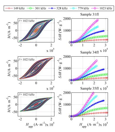
**Figure 5.** a) AC hysteresis loops of samples 31ff, 34ff and 35ff at 1023 kHz fixed frequency (left); b) *SAR* of samples 31ff, 34ff and 35ff *versus* field amplitude at different frequencies (right).
