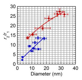
**Figure 8.** Ratio of transverse ( $r_2$ ) to longitudinal ( $r_1$ ) relaxivities at 1.41 T/60MHz (37°C) *vs.* average TEM diameters of IONPs, for nanosphere (blue) and nanoflower (red) samples. Solid lines are power law fits of exponents respectively 0.92 and 0.48.
