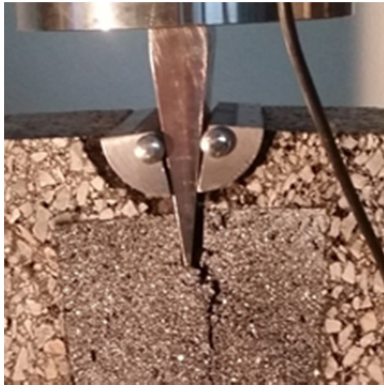
Figure 8. Wedge blocked on the bottom of the notch.
