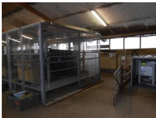
Figure M17.1. A partially open emissions measurement enclosure (source: INRA)
