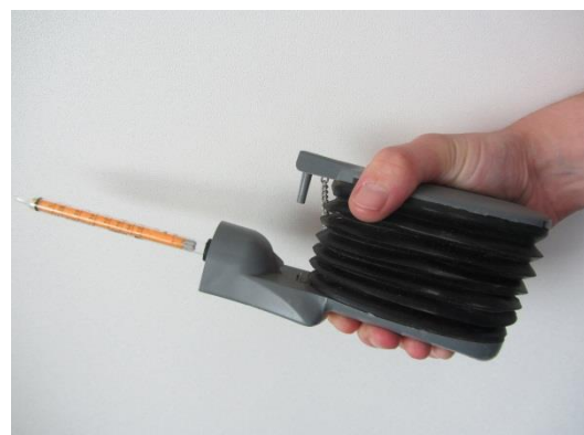
Figure M6.1. Sampling pump with colorimetric gas detector tube (source: Solène Lagadec, Brittany regional chamber of agriculture)
