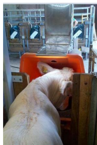
Figure M19.1. Animal feeding from a GreenFeed™ system (source: INRA)
