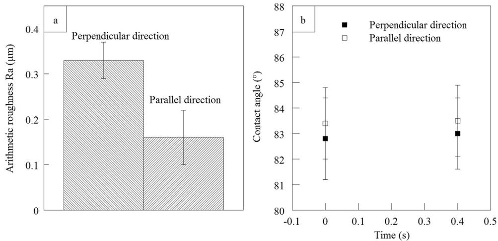
Fig. A4. (a) Arithmetic roughness  $R_a$  and (b) contact angle in relation to the direction of rolling on 1 mm rolled substrate AA 1050 degreased using acetone.
