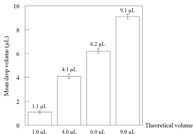
Fig. A1. Real mean drop volume deposited by the goniometer on thin glass slide for different theoretical volumes.
