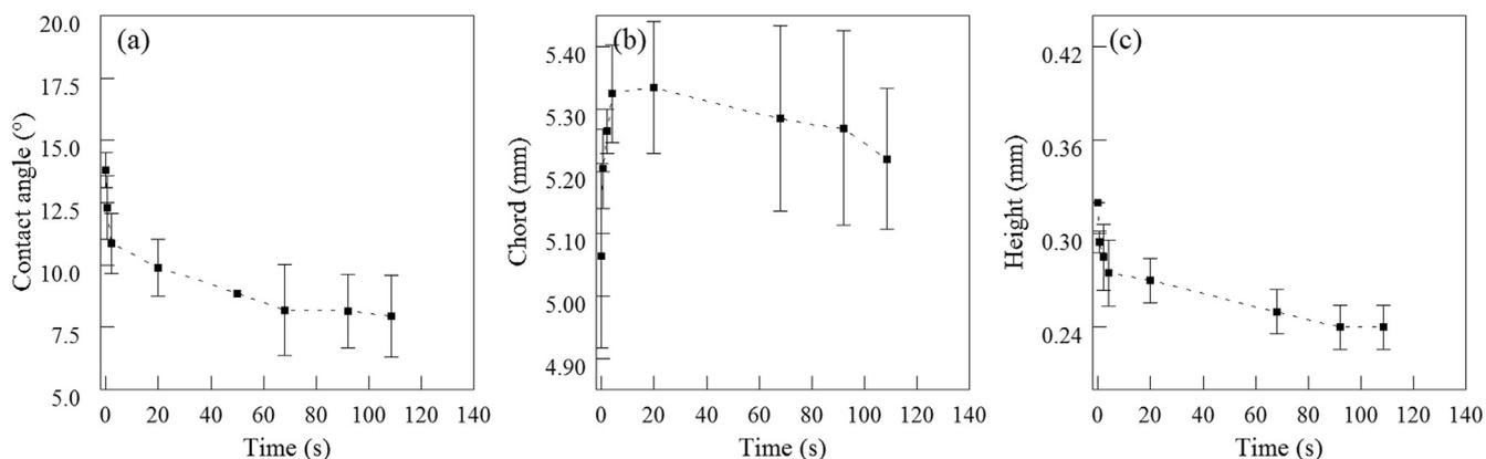
Fig. 5. Evolution of the contact angle, chord and height over time on an anodic film (5  $\mu\text{m}$ ) formed on 1 mm rolled substrate AA 2024T3.
