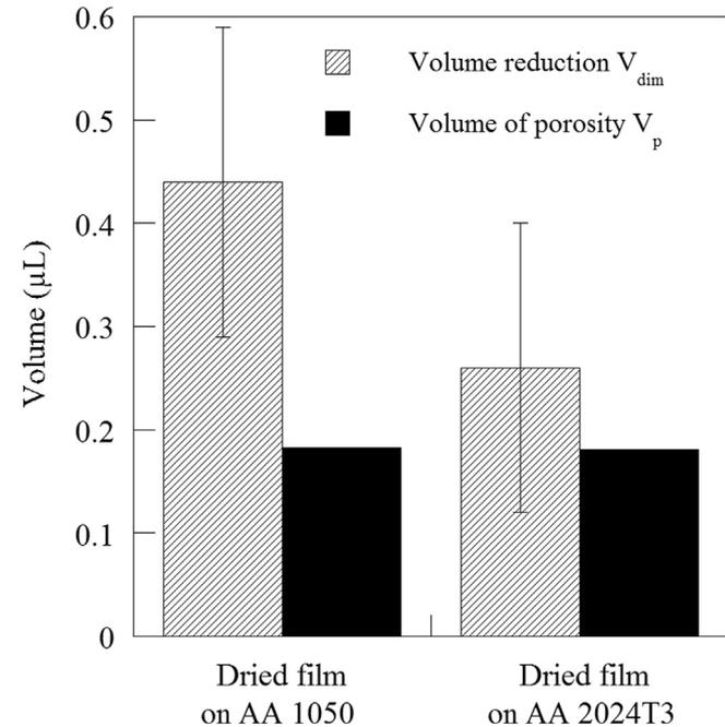
Fig. 7. Mean reduction in the drop volume ( $V_{\text{dim}}$ ) at  $t = 2$  s on anodic film ( $5 \mu\text{m}$ ) prepared on 1 mm rolled substrates AA 1050 and AA 2024. Comparison with the volume of porosity ( $V_p$ ) available in the anodic film under the surface area of the drop.
