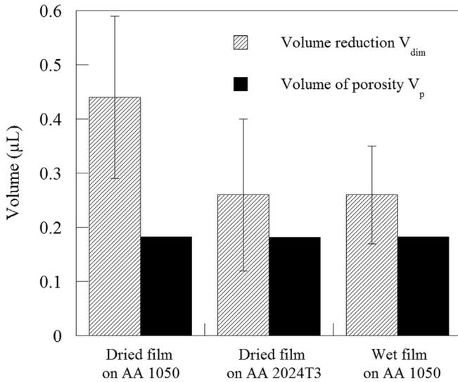
**Fig. 8.** Mean reduction in the drop volume ( $V_{dim}$ ) at  $t = 2$  s on dried anodic film (5  $\mu\text{m}$ ) on 1 mm rolled substrates AA 1050 and AA 2024 and on non-dried anodic film on 1 mm rolled substrate AA 1050. Comparison with the volume of porosity ( $V_p$ ) available in the anodic film under the surface area of the drop.
