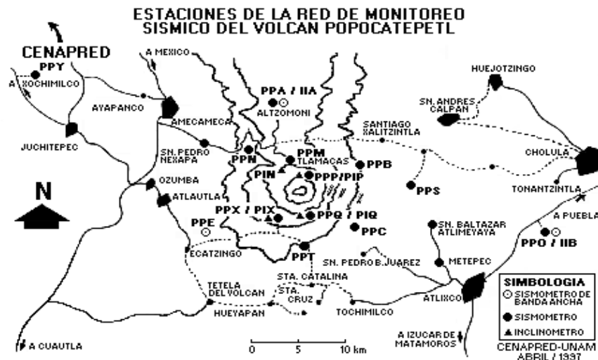
Figure 2. Measuring stations around the Popocatepetl volcano
