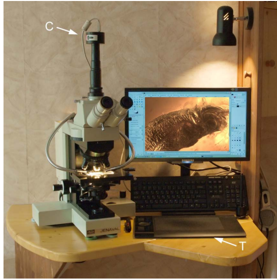
FIGURE 1: An example of a working place with the complete drawing apparatus ready to use. C-camera, T-pen tablet
