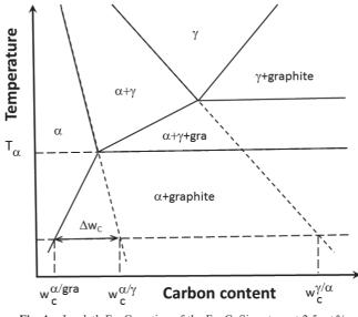
Fig. 4. Isopleth Fe–C section of the Fe–C–Si system at 2.5 wt.% Si in the stable eutectoid range.  $\Delta w_C$  shows the difference between the carbon content at the ferrite/austenite interface,  $w_C^{\alpha/\gamma}$ , and at the graphite/ferrite interface,  $w_C^{\alpha/gm}$ .
