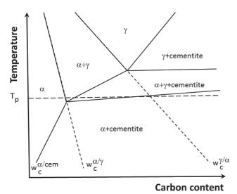
Fig. 7. Isopleth Fe–C section of the Fe–C–Si system at 2.5 wt.% Si in the metastable eutectoid range.
