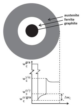
Fig. 3. Schematic of ferrite formation as halos around the graphite nodules and corresponding radial carbon distribution.  $\Delta w_C$  should be positive for carbon to diffuse to graphite from the ferrite/austenite interface to the graphite nodule.
