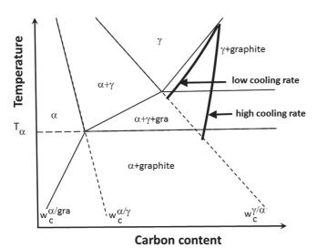
Fig. 6. Isopleth Fe–C section of the phase diagram showing the possible evolution of the average carbon content in austenite (very thick lines) during cooling at low and high cooling rate.
