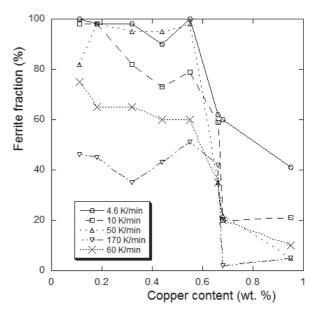
Fig. 9. Effect of copper addition on the ferrite fraction after cooling at different rates after austenitization or casting in a thermal analysis cup (60°C/min). The alloys contained 3.6–3.8 wt.% C, 2.5–2.8 wt.% Si, 0.12–0.19 wt.% Mn. After Sertucha *et al.*<sup>4)</sup>
