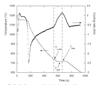
**Fig. 2.** Cooling curve and its derivative obtained by casting a standard thermal analysis cup with a nodular cast iron (3.74 C, 2.51 Si, 0.18 Mn, 0.68 Cu, wt.%) after Sertucha *et al.*<sup>4</sup> T<sub>*a*,exp</sub>, T<sub>*p*,exp</sub> and T<sub>trans</sub> are respectively the experimental temperatures for the start of the ferritic and pearlitic reactions, and for the maximum in the derivative curve.
