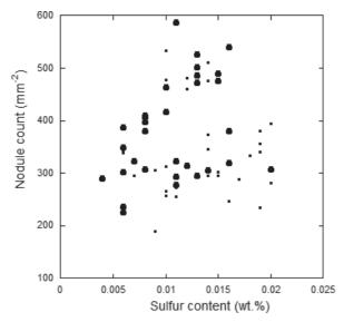
**Fig. 10.** Evolution of the nodule count N<sub>A</sub> with the sulfur content of fully ferritic (large circles) and partly pearlitic (small circles) as-cast alloys, after Sertucha *et al.*<sup>41)</sup>
