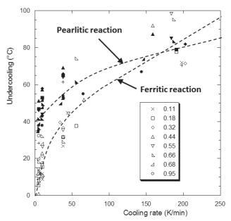
Fig. 5. Evolution with cooling rate of the start of the ferritic and pearlitic reactions measured on alloys with 3.6–3.8 C, 2.47–2.83 Si, 0.12–0.19 Mn and 0.11–0.95 Cu (indicated in the caption), in wt.%, after Sertucha *et al.*<sup>4)</sup>
