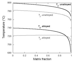
**Fig. 12.** Local reference temperatures for the ferritic and pearlitic reactions calculated along the composition profiles in Fig. 11. Both the case of an unalloyed cast iron and of an alloyed one are shown.
