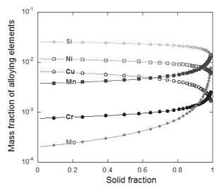
**Fig. 11.** Build-up of microsegregation of some substitutional solutes in the austenite matrix during solidification of a eutectic nodular graphite cast iron, note the logarithmic scale for plotting austenite composition. The origin of the X axis corresponds to the outer surface of nodules, *i.e.* the start of the eutectic reaction.
