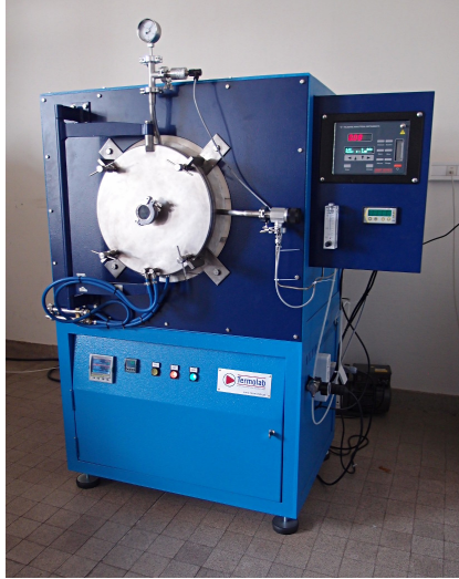
Figure 1: Chamber used for isothermal ageing at low oxygen percentage ( <0.1\% ), using an oxygen monitor and a low flow of nitrogen (0.1 standard litre per minute).
