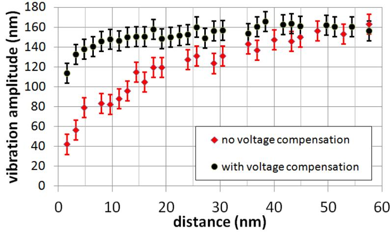
Figure 3: (color online) Amplitude of vibration recorded for a fixed excitation frequency while approaching the surface for different voltage difference. Without voltage compensation, a feedback on the amplitude will stop the approach  $\sim 20$  nm from surface with a 25% amplitude reduction set-point. With voltage compensation and identical set-point, this distance will be reduced to few nanometers.
