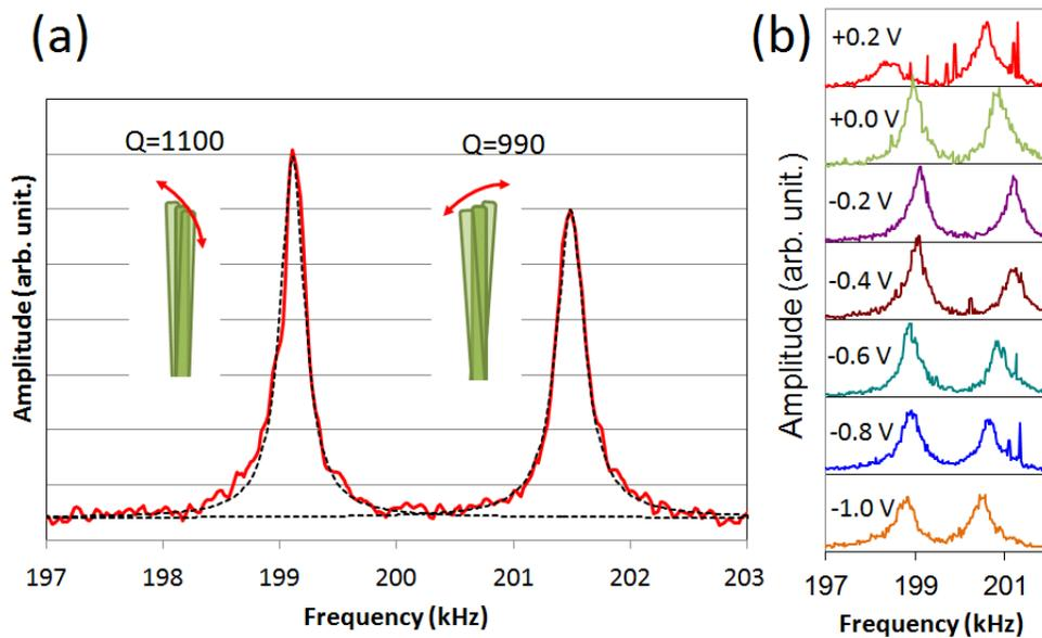
Figure 2: (color online) (a) Nanowire resonance peaks recorded far from the surface. The two perpendicular vibrations have comparable Q factors ( $\sim 1000$ ). (b) Influence of a DC voltage between tip and surface on the nanowire resonance frequency. The down-shift is a signature of electrostatic pull-in and shows that we need about  $-0.3 \pm 0.1$  V to compensate the workfunction difference.
