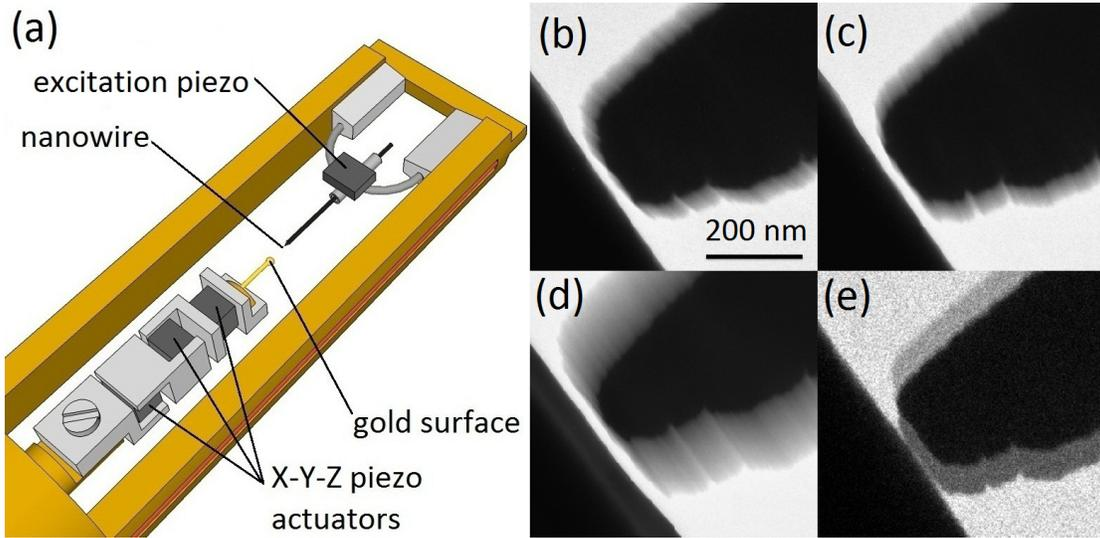
Figure 1: (color online) Experimental setup: (a) sketch of the TEM sample holder used in this study. (b) and (c) TEM images of the two nanowire vibration polarizations visible after sample holder rotation (see text). (d) Large vibration 25 nm from the surface showing the parallelism achieved on one polarization. (e) Jump to contact from video recorded at 1.5 V difference between tip and surface (see text).
