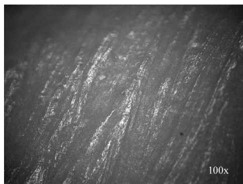
Fig. 19. Surface produced on a tool after grinding against an abradar. No lubricants used (metallographic microscope, 100x).
