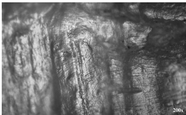
Fig. 20. Micro-wear developed on a rough surface like the one shown in figure 18 (metallographic microscope, 200x).
