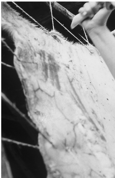
Fig. 5. Fleshing with a gouging motion. Incorrect orientation of the bevel of the tool: to effectively flesh the hide, the beveled face should be the leading face.
