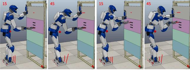
Fig. 3: Output of the PG for the pulling task of two different buttons with  $f_{\text{task}} = 15\text{N}$  and  $45\text{N}$  force. The feet are set at a fixed static position w.r.t the panel. Notice the difference in posture when the pulling force is higher and the buttons are different.
