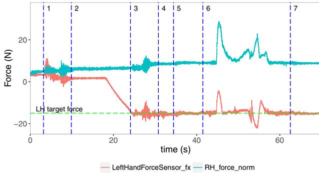
Fig. 11: The LH is controlled in admittance after phase (2) to hold a contact of  $-15\text{N}$  with the panel all along the experiment. We plotted the norm of all forces for the RH as in each step different components are used (guarded motion with its specific, putting the tool in the switch, pulling the switch and releasing it... all with different values of the desired force). These phases are clearly identifiable from the norm.
