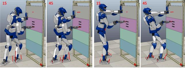
Fig. 4: Output of the PG for the pulling task of two different buttons with  $f_{\text{task}} = 15\text{N}$  and  $45\text{N}$  force. The feet positioning (floating) is determined by the PG. Notice the difference in posture and feet position when the pulling force is higher and the buttons are different.
