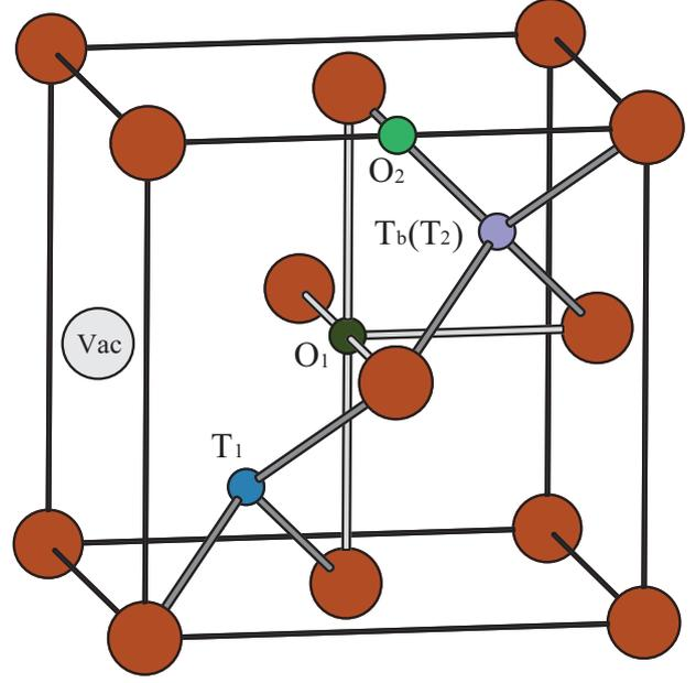
Fig. 1. Schematic representation of the interstitial sites around a vacancy (gray ball) in fcc Ni.  $O_1$  (olive green ball) and  $O_2$  (green ball) are octahedral (O) sites in first and second nearest neighbor (NN) position of the vacancy.  $T_1$  (blue ball) and  $T_2$  (violet ball) are 1NN and 2NN tetrahedral (T) sites.  $T_2$  is already considered as a bulk site, from the segregation point of view (see text).
