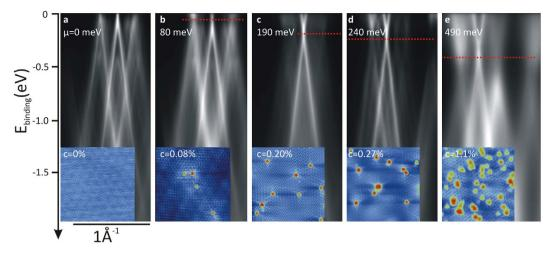
Figure 1. ARPES spectra of samples exposed for (from a to e) T=0, 7.5, 15, 30 and 90 min. The shift of the Fermi level ( $\mu = E_F - E_D$ ) is given on each spectrum. Insets are typical  $10 \times 10 \text{ nm}^2$  STM images of the corresponding samples where the nitrogen dopants appear as red protrusions; the nitrogen concentration (*c*) is given on each image.
