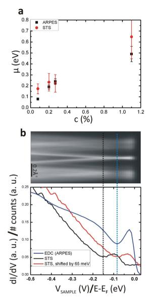
**Figure 4.** (a)  $\mu$  for each sample measured with STS (red) and with ARPES (black). (b) ARPES spectrum taken on the lightly-doped sample (c = 0.08% and  $\mu = 80$  meV). Graph: comparison between STS and EDC data (extracted from the ARPES spectrum) revealing the importance of taking into account the apparent gap around the Fermi level in the tunneling spectra.
