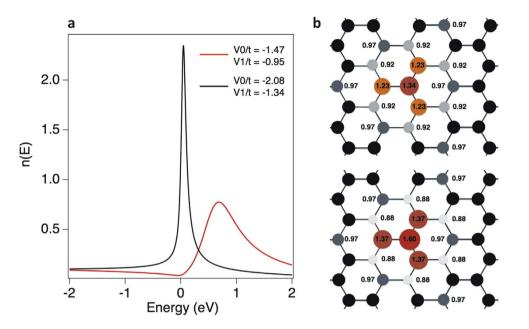
**Figure 6.** (a) Local density of states on the nitrogen atom for two sets of extended potentials defined by  $V_0$  on the nitrogen atom and  $V_1$  on the first neighbors. (b) Mulliken  $\pi$  charges around the nitrogen impurity: (top)  $V_0/t = -1.47$ ,  $V_1/t = -0.95$  (corresponding to the red curve in a); (bottom)  $V_0/t = -2.08$ ,  $V_1/t = -1.34$ ; t = 2.72 eV (corresponding to the black curve in a).
