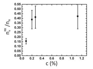
Figure 5. Charge transfer per nitrogen dopant (according to the rigid band model) determined from the ARPES data.
