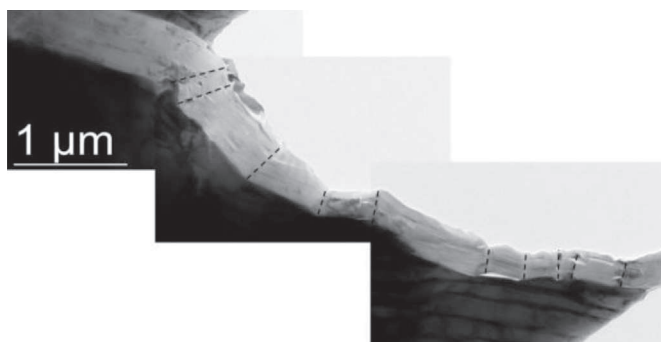
Fig. 10. Bright field TEM image of a graphite flake showing successive segments of different orientations along the length of the flake.
