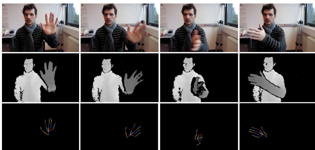
Figure 2: Example of a swipe left gesture represented in color (top), depth map (middle) and skeletal data (bottom).
