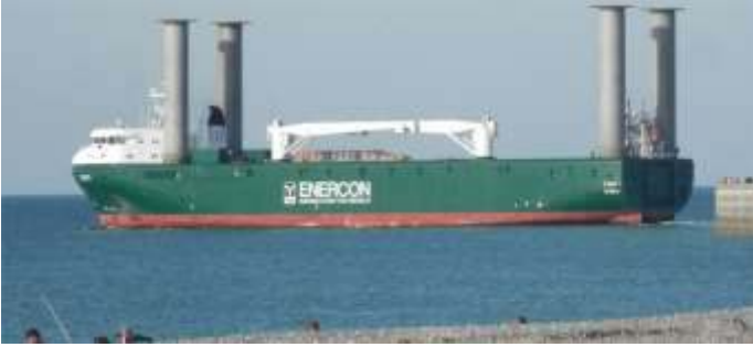
FIGURE 6: PHOTO OF THE ROLO CARGO E-SHIP 1 EQUIPPED WITH 4 FLETTNER ROTORS [9].
