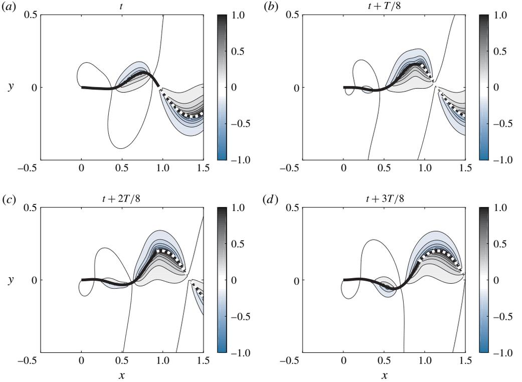
FIGURE 2. (Colour online) Flow created in the midplane  $z=0$  during a flapping sequence for  $M^* = 10$ ,  $U^* = 20$  and  $H^* = 0.1$ . Instantaneous normalized velocity potential obtained from (3.2) and (3.3) using a frozen wake model of non-dimensional length  $L_w = 2$ . The flag's (respectively wake's) position is shown by a thick black (respectively dashed) line.
