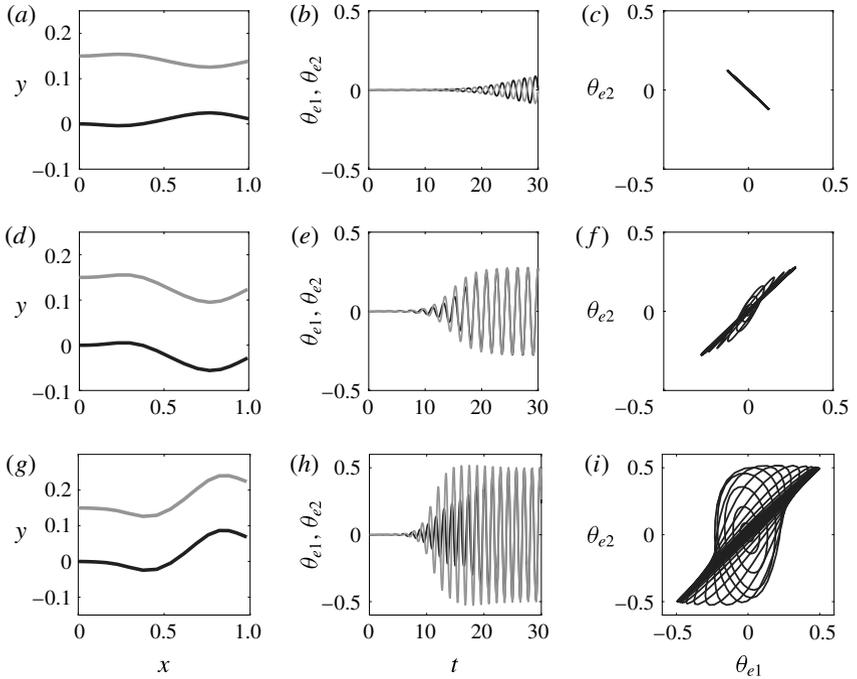
FIGURE 7. Flapping dynamics for  $H^* = 0.1$ ,  $d^* = 0.15$ ,  $M^* = 27$  and  $U^* = 9$  (a-c),  $U^* = 10$  (d-f) and  $U^* = 11.7$  (g-i). (a,d,g) Show the flags' instantaneous position. (b,e,h) and (c,f,i) Show the evolution of trailing edge angles  $\theta_{ei}$ .
