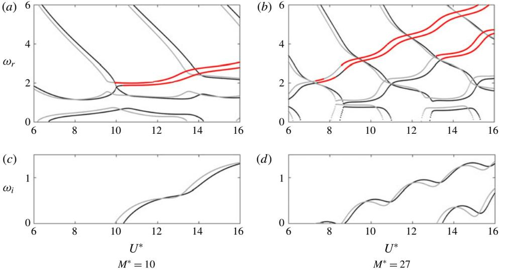
FIGURE 4. (Colour online) Frequencies (a,b) and growth rates (c,d) for  $H^* = 0.1$  and  $d^* = 0.15$ . The black lines (respectively grey lines) correspond to in-phase (respectively out-of-phase) modes. Frequencies corresponding to positive growth rates are shown in bold red.
