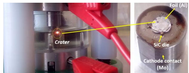
Fig. 15. Picture showing the location of the contact responsible for current conduction (10 A) after failure. Despite the low contact resistance ( \sim 100\text{ m}\Omega ), the small size of the contact area ( \sim 0.1\text{ mm}^2 ) results in a very high power density, hence the light emission.
