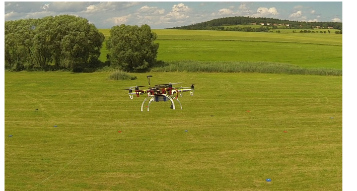
Fig. 3: The hexarotor UAV used during the experimental verification of the proposed RDTSP in scenario with initial plan obtained as the DTSP (for more details see http://mrs.felk.cvut.cz/ecmr17rdtsp )
