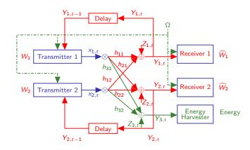
Fig. 1. Two-user Gaussian interference channel with a non-collocated energy harvester.
