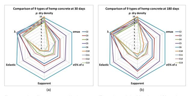
Fig. 5: comparison of hemp concretes taking into account different characteristics, (a) 30 days and (b) 180 days.
