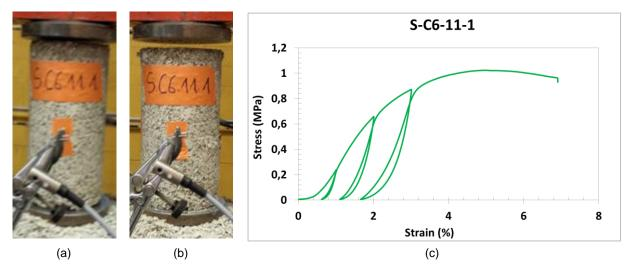
Fig. 4: mechanical response: medium deformation, specimen before (a) and after (b) test with stress-strain curve (c) [NIY 17].
