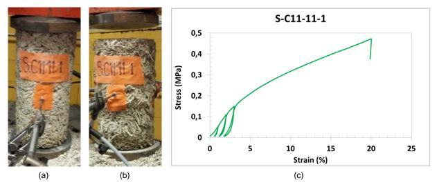
Fig. 2: mechanical response: high deformation, specimen before (a) and after (b) test with stress-strain curve (c) [NIY 17].
