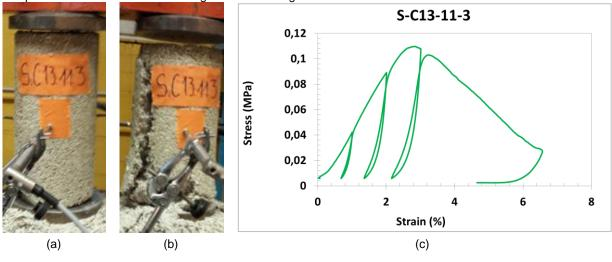
Fig. 1: mechanical response: low deformation, specimen before (a) and after (b) test with stress-strain curve (c) [NIY 17].
