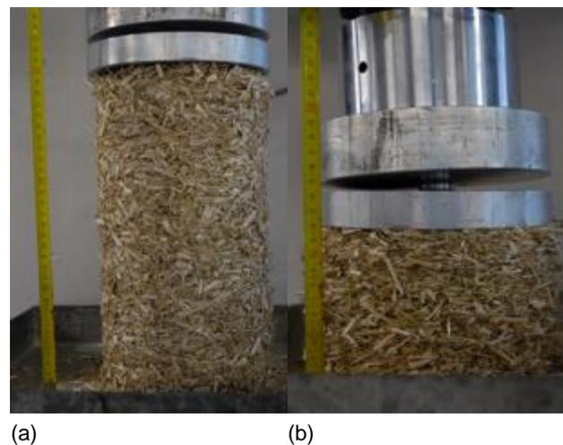
Fig. 3: hemp particles mechanical response, before (a) and after (b) compression test [GOU 14].
