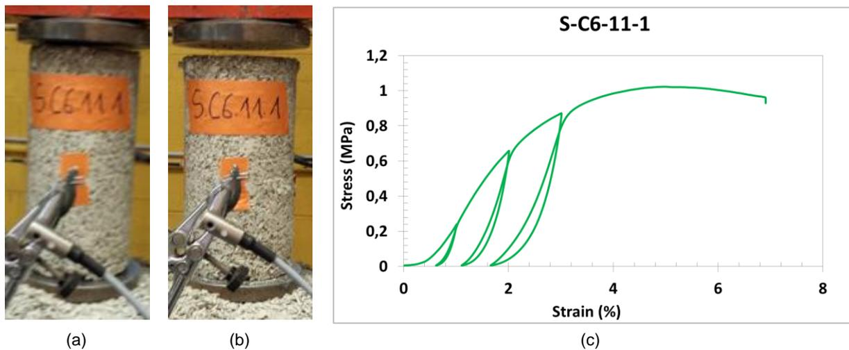
Fig. 4: mechanical response: medium deformation, specimen before (a) and after (b) test with stress-strain curve (c) [NIY 17].
