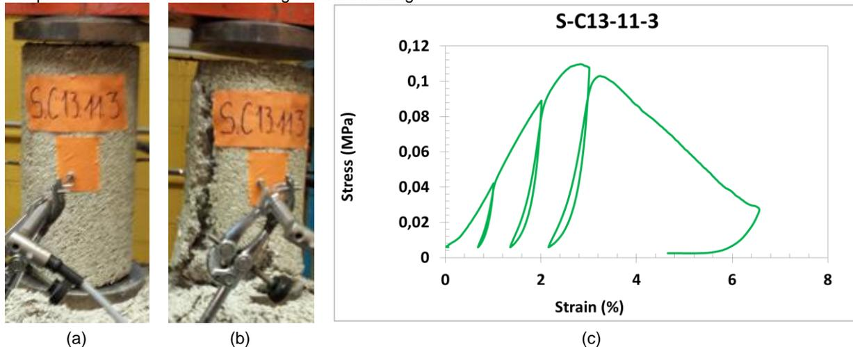
Fig. 1: mechanical response: low deformation, specimen before (a) and after (b) test with stress-strain curve (c) [NIY 17].
