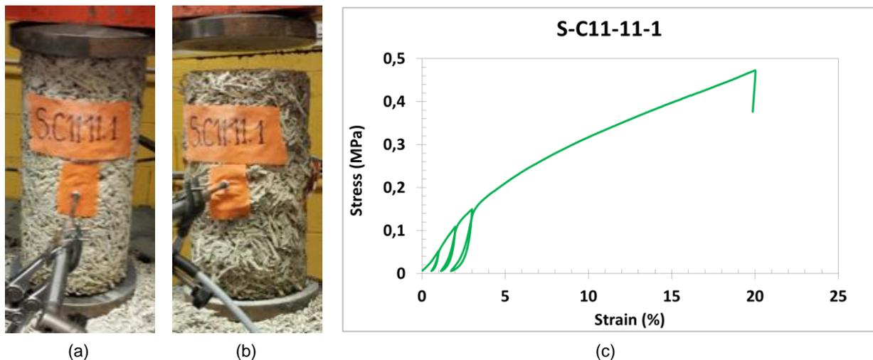
Fig. 2: mechanical response: high deformation, specimen before (a) and after (b) test with stress-strain curve (c) [NIY 17].
