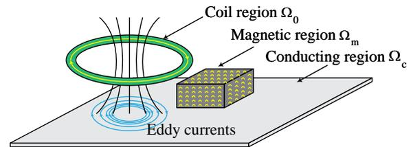
Fig. 1. Illustration of a magnetodynamic problem with coils, magnetic regions and conductive region.
