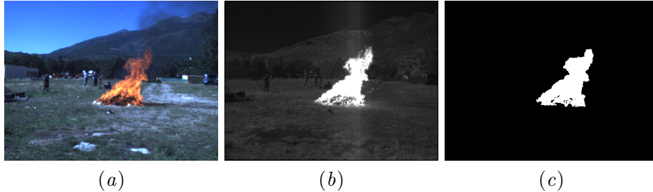
Figure 1: Example of images of the database taken with the multi-spectral camera. (a) image of the visible spectra, (b) image of the near infrared spectra and (c) ground truth based on the image (a).
