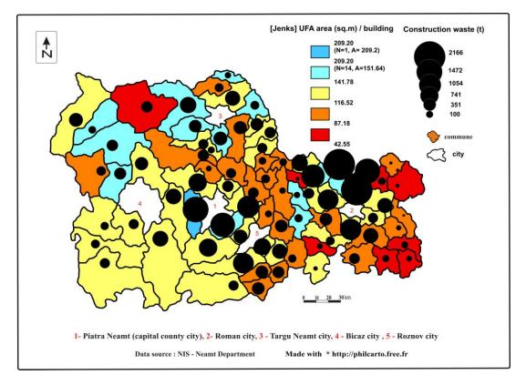
Figure 3. Construction waste generated by the new residential buildings in rural areas
