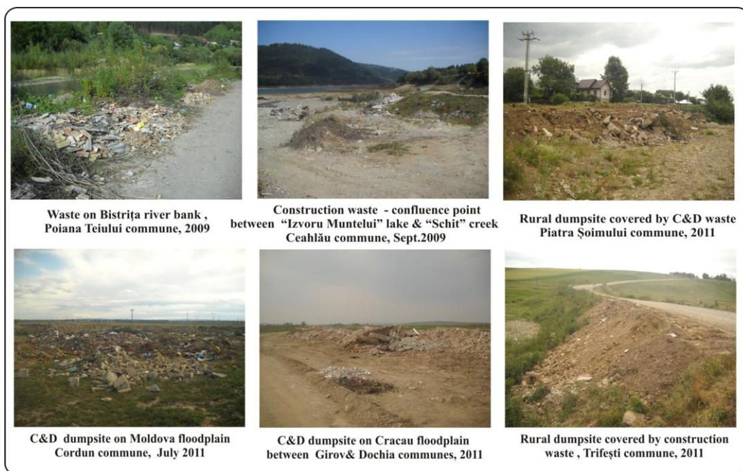
**Figure 5.** Uncontrolled waste disposal of CDW waste in rural areas and reuse of this fraction as coating material for local dumpsites
