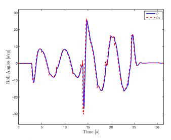
**Fig. 16** Attitude and reference for  $\phi$  angles in case 1.
