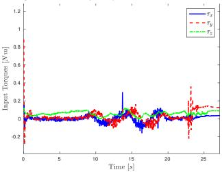
Fig. 46 Quad-rotor's experiment control torques for case 1.
