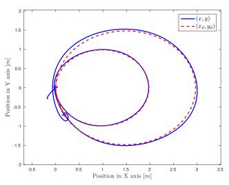
Fig. 31 Quad-rotor's horizontal translation in case 2 experiments.
