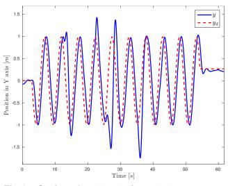
Fig. 73 Quad-rotor's position in the y axis in case 2.
