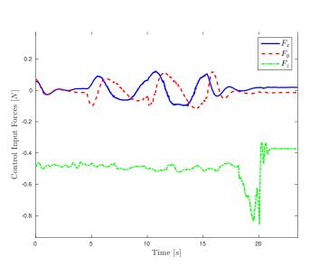
Fig. 33 Quad-rotor's control forces for case 2.
