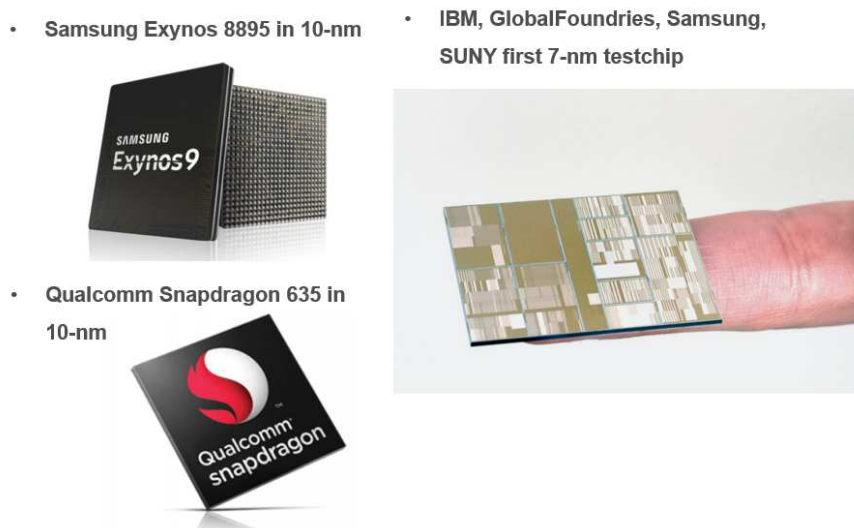
Figure 3: Examples of 10-nm processors and prototype 7-nm circuit by IBM
