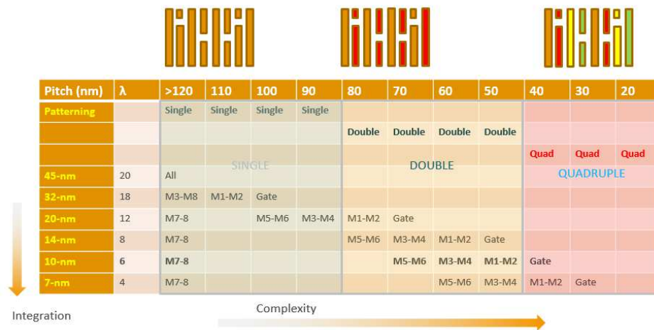
Figure 23: Single, double and quadruple patterning as a function of interconnect pitch [Brain2017]
