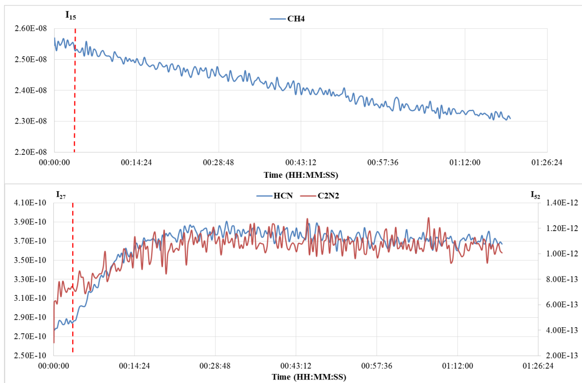
Figure 11. Time-monitoring mass spectrum in MID mode following the consumption of the reactive \text{CH}_4 (top) and the production of the HCN and \text{C}_2\text{N}_2 molecules (bottom). The red dotted lines mark the beginning of the irradiation of the APSIS reactor with the VUV source.
