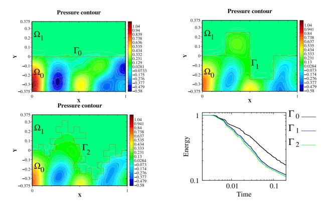
Figure 3: Pressure contours at t = 0.01 in cavities with an internal boundary of different Minkowski fractal generations (from left to right and top to bottom:  $\Gamma_0$  (flat),  $\Gamma_1$  and  $\Gamma_2$ ) and the corresponding energy damping. The size of the mesh is  $128 \times 512$ .
