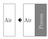
Figure 1: One medium for the absorption on the boundary (left) and two media for the absorption in the volume (right).
