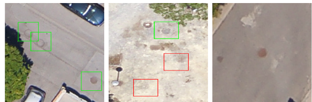
Figure 5. Examples of detected manholes covers, false positives and non detected manhole covers by the customized network. Green boxes correspond to detected manholes covers, red boxes to false positives.
