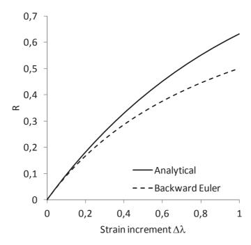
Fig. 1 – Influence of the increment size on the accuracy of the time integration of Voce's isotropic hardening equation. Parameters  $R_{sat} = C_R = 1$  were used.
