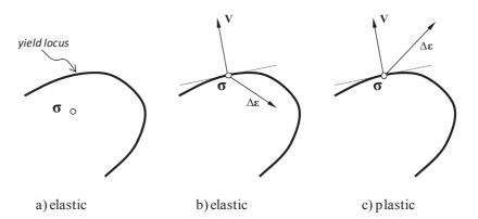
Fig. 2 – Schematic illustration of loading–unloading conditions in the framework of an explicit time integration algorithm, given a stress state  $\sigma$  and a loading increment  $\Delta \varepsilon$ .
