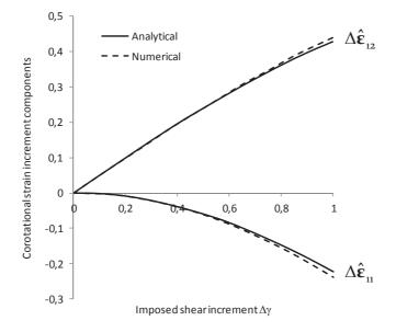
Fig. 3 - Influence of the increment size on the accuracy of the co-rotational strain increment.
