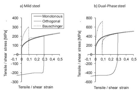
Fig. 4 – Rheological simulation of monotonic shear, reverse shear (Bauschinger) and tension followed by shear in the same direction (Orthogonal). Material parameters from [30] corresponding to two classical forming steel grades.
