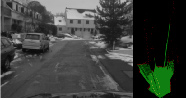
Fig. 5. An evidential grid created using a Lidar 4 nappes. The green color shows the free cells, the red shows the occupied cells and the black represents unexplored cells (unknown). The yellow circle includes a error detection because of snow on the Lidar .
