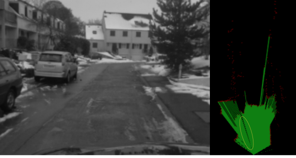
Fig. 5. An evidential grid created using a Lidar 4 nappes. The green color shows the free cells, the red shows the occupied cells and the black represents unexplored cells (unknown). The yellow circle includes a error detection because of snow on the Lidar .
