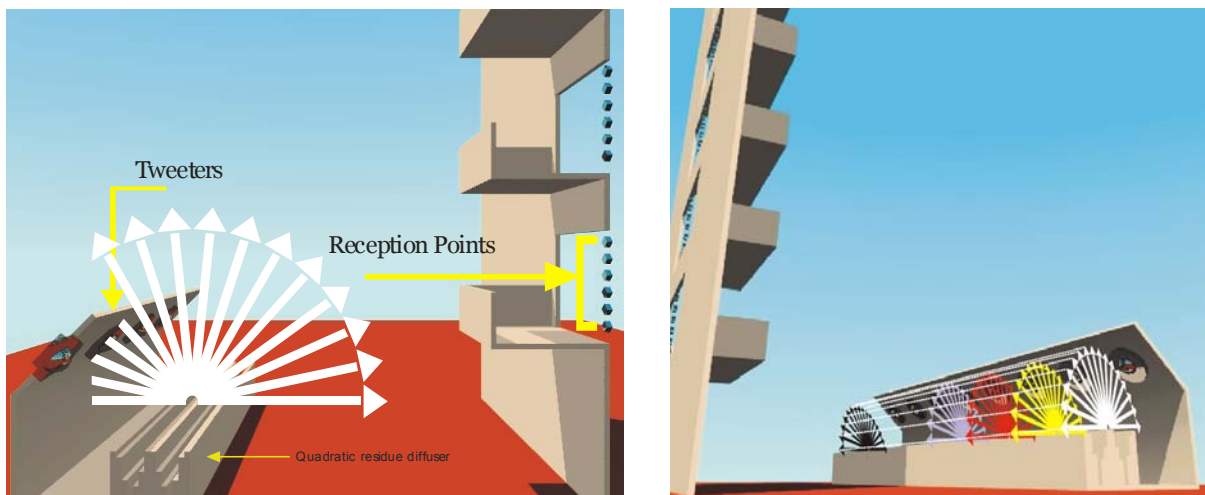
Fig. 5. Line source with a quadratic residue diffuser.
